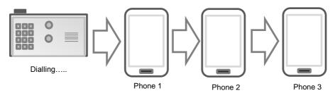
Any user receiving the call can answer, speak to the visitor, and press the following digits on their mobile or fixed line telephone to control the relay on the device...
