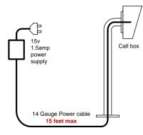
**Tip:** 18 gauge cable will not run the unit. You may experience various issues with performance if the power cable is more than 15 feet and using thin cable such as 18 gauge.
